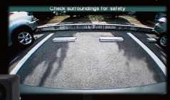
The Rear View Camera allows you to see blind spots behind a vehicle by automatically projecting its rear view on the display whenever the gear is in reverse.
